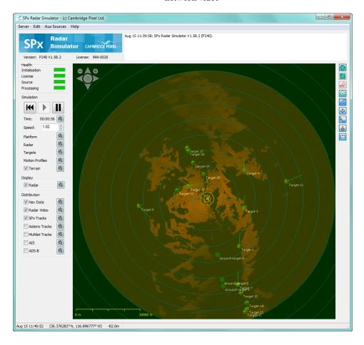
Figure 3 - Cambridge Pixel's SPx Simulator generates simulated ASTERIX CAT-240 video along with terrain, targets and representative system noise.
