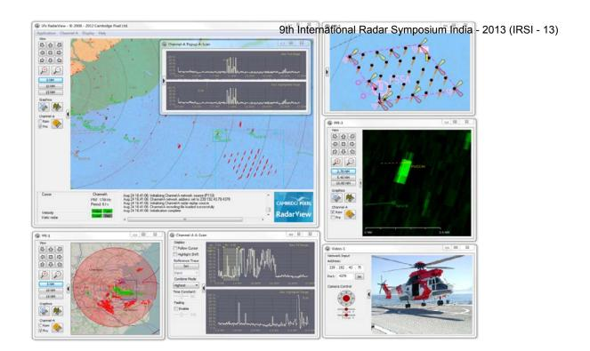
Figure 2 - Display of radar video received from a Kelvin Hughes SharpEye radar using ASTERIX CAT-240 network video
